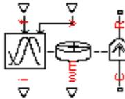
The Piezo Rotary Motor block represents the torque-speed characteristics of a piezoelectric traveling wave motor. The block represents the torque-speed relationship of the motor at a level that is suitable for system-level modeling. To simulate the motor, the block uses the following models:
