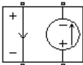
The PCCCS (Polynomial Current-Controlled Current Source) block represents a current source whose output current value is a polynomial function of the current through the input ports. The following equations describe the current through the source as a function of time:
