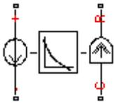
The Generic Rotary Actuator block implements a model of a generic rotary actuator designed to be driven from a DC voltage source or PWM driver. You define torque-speed characteristics in terms of tabulated values for powering the motor at the rated voltage. This functionality allows you to model a motor without referencing an equivalent circuit.
