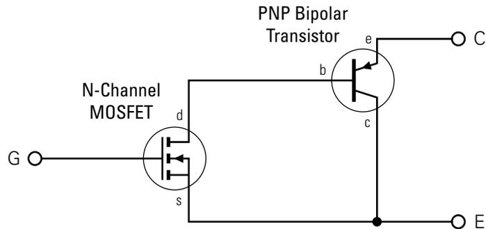
The MOSFET source is connected to the bipolar transistor collector, and the MOSFET drain is connected to the bipolar transistor base. The MOSFET uses the equations shown in the N-Channel MOSFET block reference page. The bipolar transistor uses the equations shown in the PNP Bipolar Transistor block reference page, but with the addition of an emission coefficient parameter  $N$  that scales  $kT/q$ .
