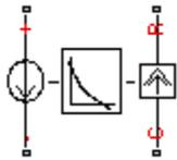
The Generic Linear Actuator block implements a model of a generic linear actuator designed to be driven from a DC voltage source or a PWM driver. Define force-speed characteristics in terms of tabulated values for powering the motor at the rated voltage. This functionality enables you to model a motor without referencing an equivalent circuit.
