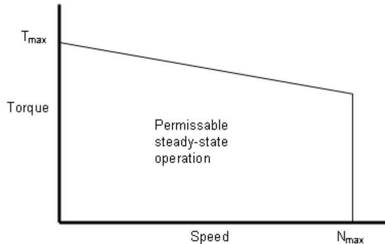
Specify the torque-speed envelope for the forward-direction motoring region (Quadrant 1) only. This region is typically the only one specified by manufacturers. The Servomotor block implements this torque-speed envelope regardless of motor direction or power flow direction, interpreting the x-axis as the absolute value of speed and the y-axis as the absolute value of torque.
