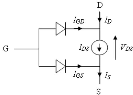
G is the transistor gate, D is the transistor drain and S is the transistor source. The drain-source current,  $I_{ds}$ , depends on the region of operation and whether the transistor is operating in normal or inverse mode.
