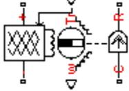
The Servomotor block represents a brushless motor with closed-loop torque control. This block abstracts the torque-speed behavior of the combined motor and motor driver in order to support system-level simulation where simulation speed is important.
