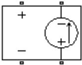
The PVCCS (Polynomial Voltage-Controlled Current Source) block represents a current source whose output current value is a polynomial function of the voltage across the input ports. The following equations describe the current through the source as a function of time:
