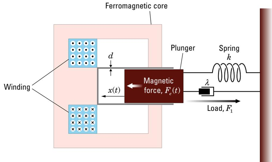
The return spring is optional. To remove the effects of this spring from the model, set the **Spring constant** parameter to 0.
