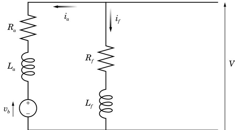
When you set the **Model parameterization** parameter to **By equivalent circuit parameters**, you specify the equivalent circuit parameters for this model:
