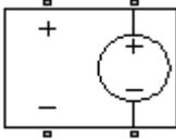
The PVCVS (Polynomial Voltage-Controlled Voltage Source) block represents a voltage source whose output voltage value is a polynomial function of the voltage across the input ports. The following equations describe the voltage across the source as a function of time:
