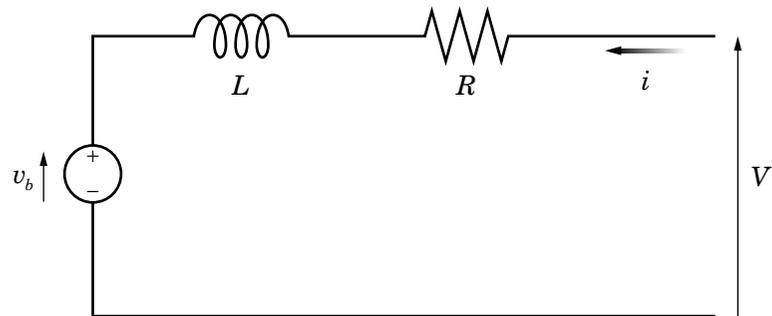
You specify the equivalent circuit parameters for this model when you set the **Model parameterization** parameter to **By equivalent circuit parameters**. The resistor  $R$  corresponds to the resistance you specify in the **Armature resistance** parameter. The inductor  $L$  corresponds to the inductance you specify in the **Armature inductance** parameter. The permanent magnets in the motor induce the following back emf  $v_b$  in the armature:
