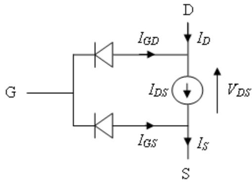
G is the transistor gate, D is the transistor drain and S is the transistor source. The drain-source current,  $I_{ds}$ , depends on the region of operation and whether the transistor is operating in normal or inverse mode.
