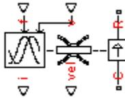
The Piezo Linear Motor block represents the force-speed characteristics of a linear piezoelectric traveling wave motor. The block represents the force-speed relationship of the motor at a level that is suitable for system-level modeling. To simulate the motor, the block uses the following models:
