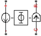
The FEM-Parameterized Rotary Actuator block implements a model of a rotary actuator defined in terms of magnetic flux. Use this block to model custom rotary actuators and motors where magnetic flux depends on both rotor angle and current. You parameterize the block using data from a third party Finite Element Magnetic (FEM) package.
