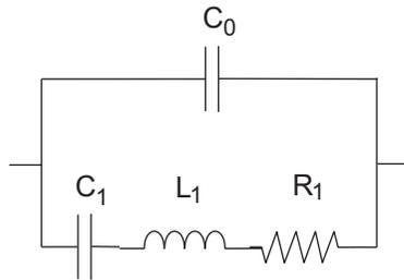
You specify the equivalent circuit parameters for this model when you set the **Parameterization** parameter to **Equivalent circuit parameters**.
