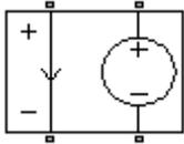
The PCCVS (Polynomial Current-Controlled Voltage Source) block represents a voltage source whose output voltage value is a polynomial function of the current through the input ports. The following equations describe the voltage across the source as a function of time:
