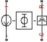
The FEM-Parameterized Linear Actuator block implements a model of a linear actuator defined in terms of magnetic flux. Use this block to model custom solenoids and linear motors where magnetic flux depends on both distance and current. You parameterize the block using data from a third party Finite Element Magnetic (FEM) package.
